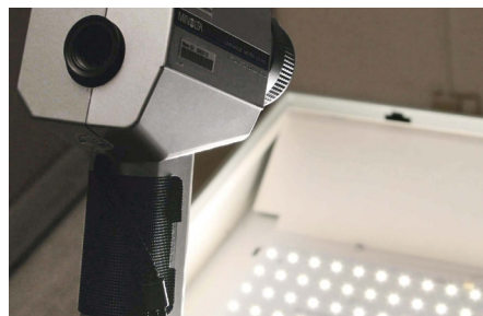
Durable high reflectance powder coat paint is applied after fabrication and reflectivity is tested.
